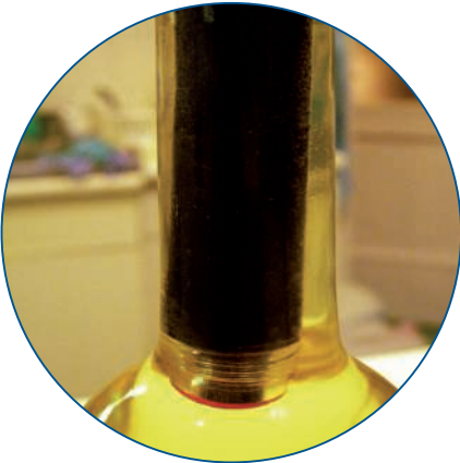
Figs. 3 und 4: Oxygen measurement in a bottle with HQD and LDO sensor
